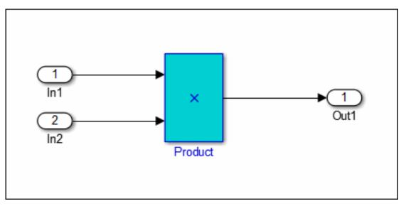
**2** Examine the model. The highlighted block multiplies two full-range signals, which could result in an overflow.
